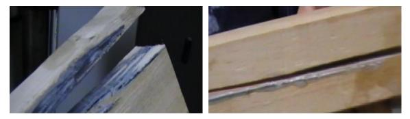
Fig. 2 Middle reinforcement application: one sheet of composite material
